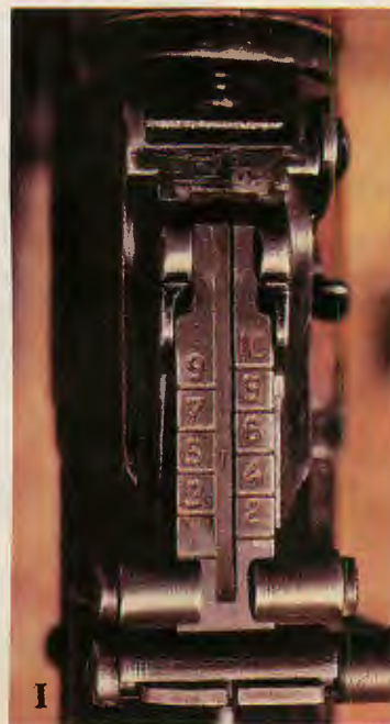
I: Tangent rear sight with open notch adjustable for elevation out to 1,000 meters. H: Forty-round RPK-74 glass-reinforced plastic magazine.
